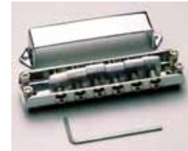
To raise the height of the strings from the surface of the neck, raise the bridge by turning each of the four adjusting screws clockwise using the adjusting key supplied with the instrument. Lower the playing action by turning the adjusting screws counterclockwise.
