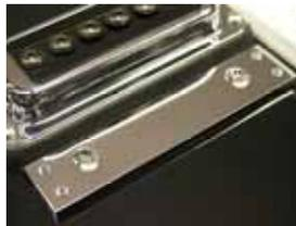
closer to the tail of the instrument while round wound strings favor a position toward the neck. Carefully re-tighten the baseplate before restringing.
